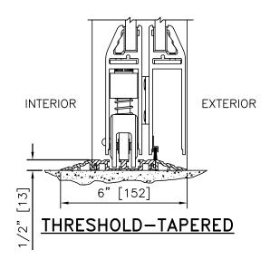
NOTE: THRESHOLDS ARE NOT REQUIRED ON THE 2000 SERIES, HOWEVER, DUE TO VARIOUS FLOORING CONDITIONS THE THRESHOLDS SHOWN ARE AVAILABLE.
